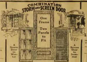
This convenient double duty door is made of Clear White Pine—strong, durable, well built throughout, 1½ inches thick. Screen panel is covered with best grade galvanized wire cloth. Storm panel glazed with good quality clear plain glass. Doors are ¾ inch longer than sizes listed to allow for drop in sill. Furnished in the "white"—not painted or varnished.
